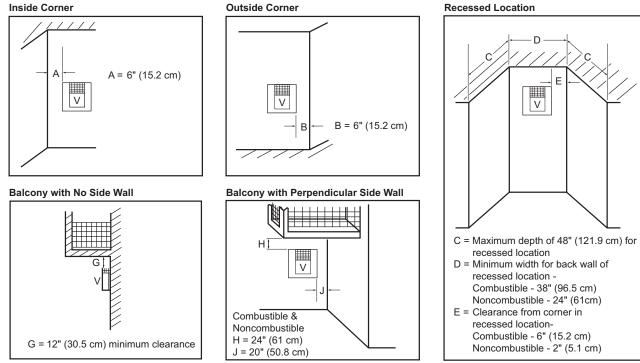
Figure 7 - Minimum Clearances for Termination Cap
